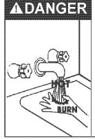
Water temperature over 125°F (52°C) can cause severe burns instantly resulting in severe injury or death.
